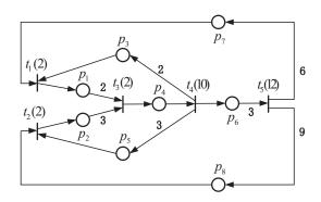
Fig. 2. The TWMG model of an assembly line.
