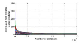
Fig. 2. Evolution of the estimated lower bound on the optimal execution time  $F(Y^*)$  computed as  $\frac{\hat{c}_{ave,i}}{\hat{\gamma}_{ave,i}}$  by each node.
