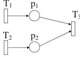
Fig. 1. Example of a Continuous Petri Net
