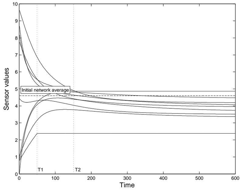
Fig. 4. Evolution of a sensor network with multiple "stuck at" faults.
