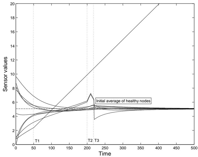
Fig. 7. Evolution of a sensor network with single "ramp" fault when the fault recovery procedure is implemented.
