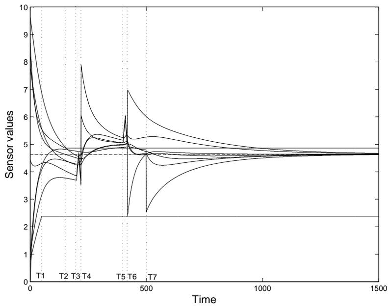
Fig. 5. Evolution of a sensor network with multiple "stuck at" faults when the fault recovery procedure is implemented.
