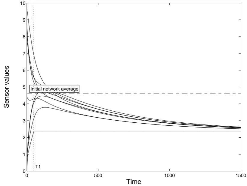
Fig. 2. Evolution of a sensor network with a single "stuck at" fault.
