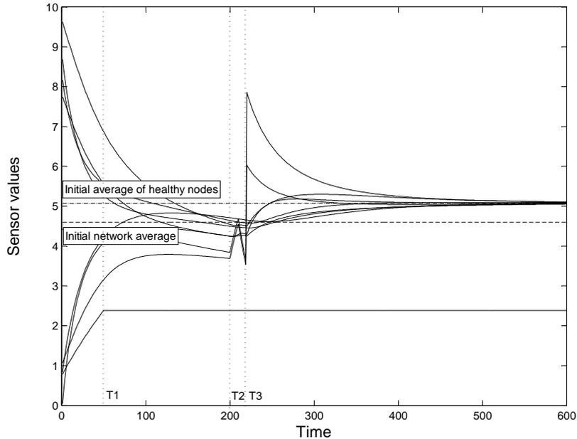
Fig. 3. Evolution of a sensor network with a single "stuck at" fault when the fault recovery procedure is implemented.
