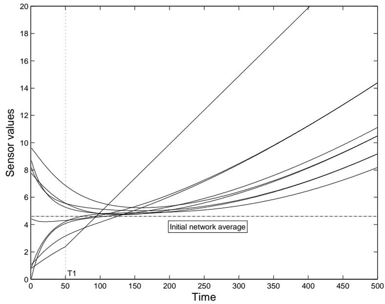
Fig. 6. Evolution of a sensor network with single "ramp" faults.
