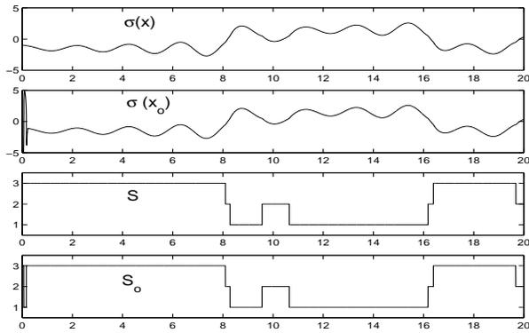
Fig. 7 : Switching surfaces  $\sigma(x)$  and  $\sigma(\tilde{x})$ , and switching indicators  $S$  and  $S_0$
