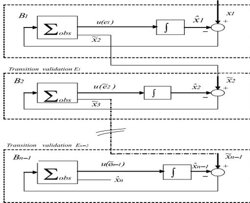
Fig. 3 : Structure of step by step differentiator
