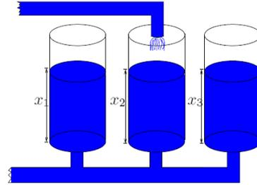
Fig. 4. Tanks System – Switched inflow
