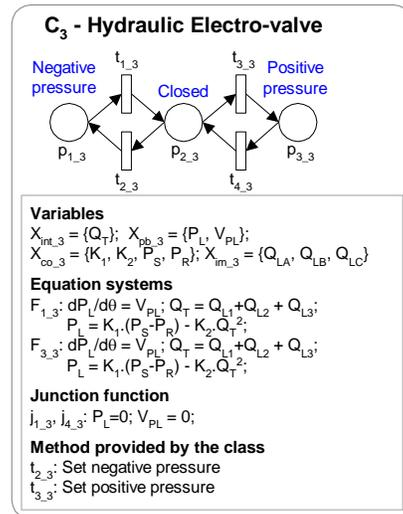
Figure 6. OO-DPT net of class  $C_3$  - Hydraulic Electro-valve.
