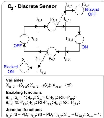
Figure 5. OO-DPT net of class  $C_2$  - Discrete Sensor
