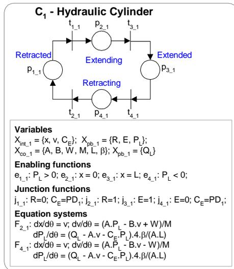
Figure 2. OO-DPT net of class  $C_1$  – Hydraulic Cylinder.
