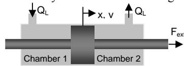
Figure 1. Hydraulic Cylinder.
