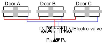
Figure 4. Door hydraulic circuit.
