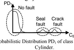
Figure 3. Probabilistic Distribution  $PD_1$  of class  $C_1$  – Hydraulic Cylinder.
