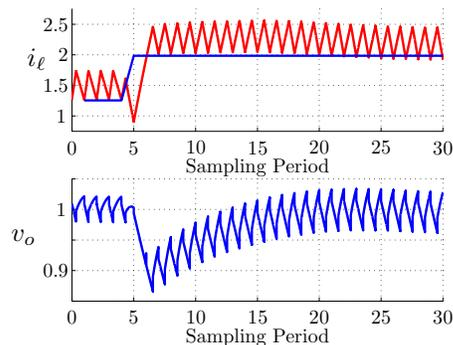
(a) Inductor current (above, with reference) and output voltage (below), in p.u.
