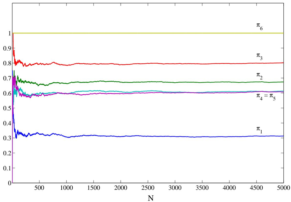
Figure 4: Computation of the node activation probabilities by simulation for the network in Example 3.
