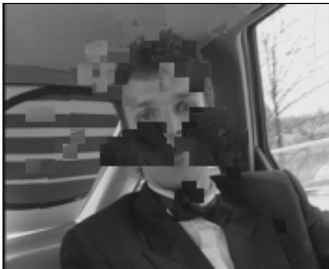
**Fig. 4: Errors due to wrong interpolation.** Sometime, especially on high ratio video sequences, motion vector leads to wrong positioning. This must be taken in consideration and a motion compensation algorithm for interpolated vectors should be adopted.
