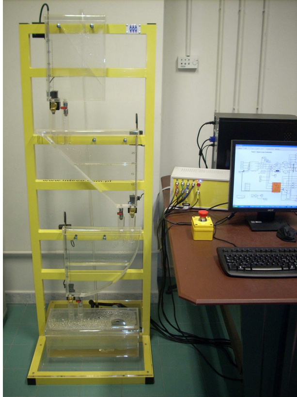
Fig. 8. The laboratory-size three-tank system
