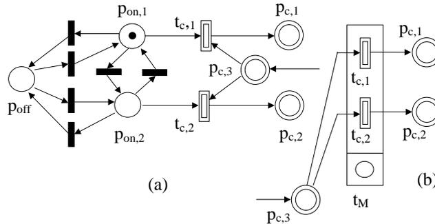
Figure 6: *The Petri net model of a machine that fills bottles: (a) detailed representation, (b) simplified representation.*
