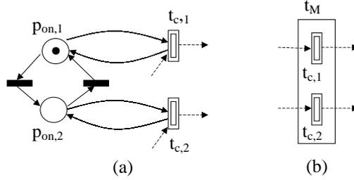
Figure 3: *The Petri net model of a macro transition: (a) detailed representation, (b) simplified representation.*
