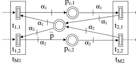
Figure 7: *The simplified Petri net model of a buffer.*
