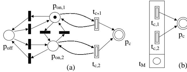
Figure 5: *The Petri net model of a machine that produces bottles: (a) detailed representation, (b) simplified representation.*
