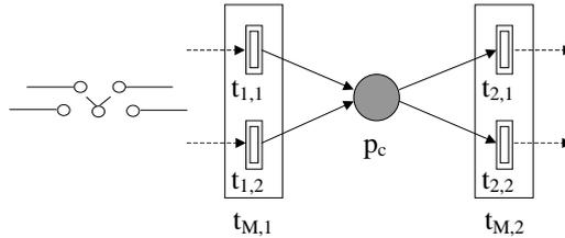
Figure 4: *A MIMO switch with 2 input and 2 output lines.*
