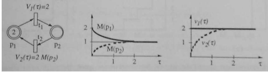
Figure 5: A timed continuous Petri net with variable maximal firing speeds.
