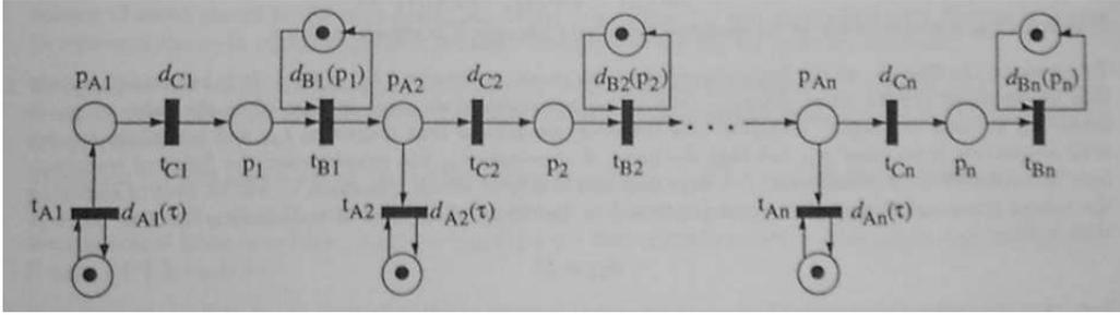
Figure 7: Discrete Petri net model of a canal with  $n$  reaches.
