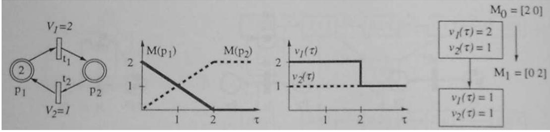
Figure 4: A timed continuous Petri net with constant maximal firing speeds.
