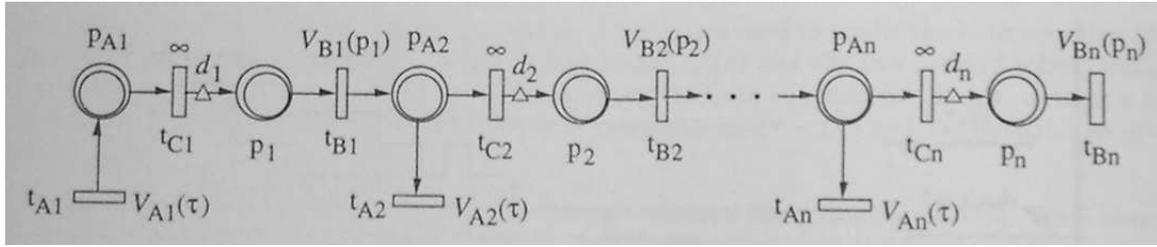
Figure 9: Timed continuous Petri net model of a canal with  $n$  reaches.
