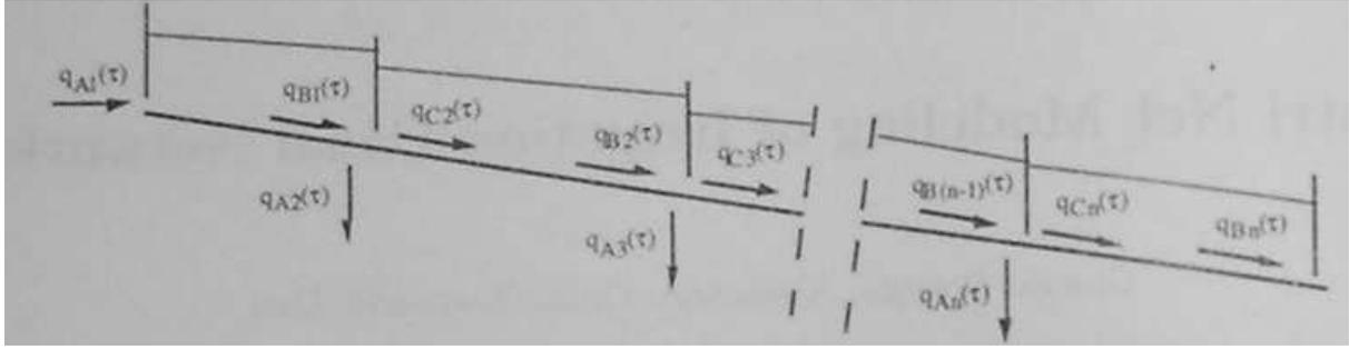
Figure 1: A canal network with  $n$  cascaded reaches.
