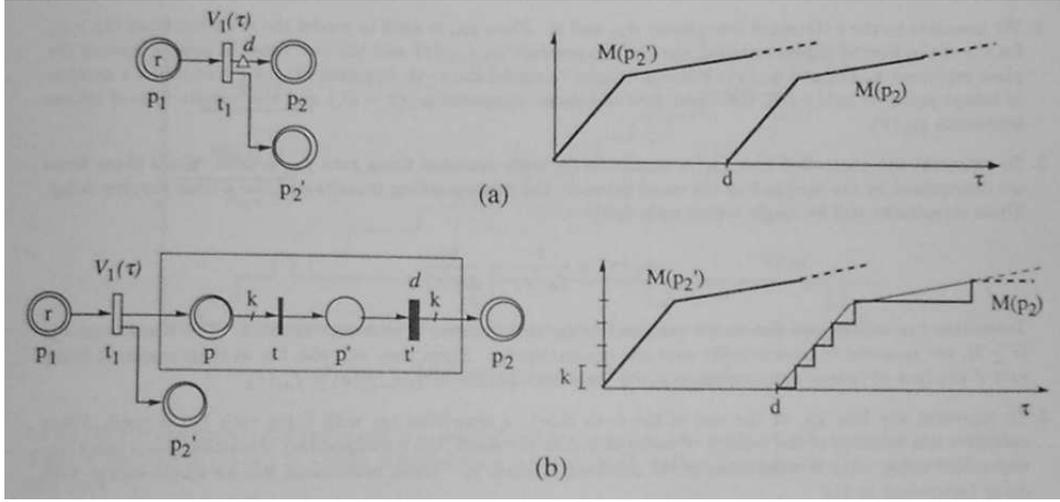
Figure 6: (a) A continuous transition with delay arc. (b) Equivalent structure.
