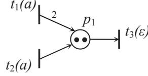
Figure 2. An LPNO that cannot be converted into an LPN.
