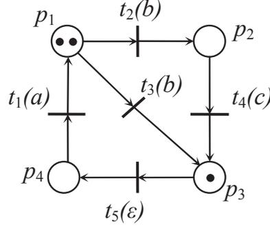
Figure 1. An LPNO with linear observation function.
