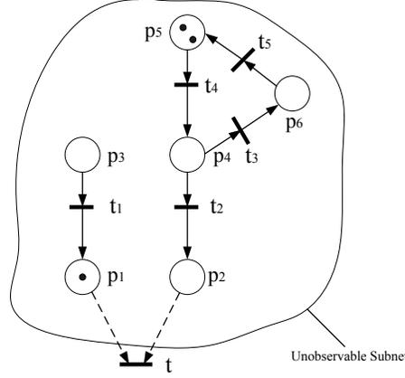
Fig. 1. Unobservable subnet with cycles.
