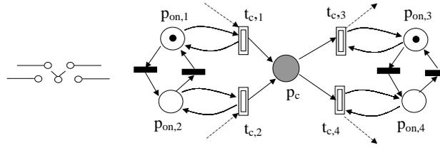
**Fig. 1.** A MIMO switch with 2 input and 2 output lines.
